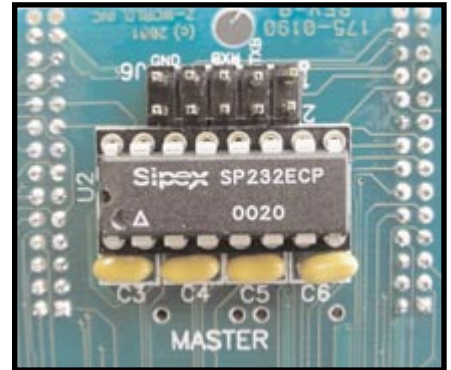
Photo 6 —I added this SipeX 232 RS-232 converter IC to initially test the upgrade module's serial port design. The RCM2300 Development Kit has provisions for this addition. All you have to do is add the parts.
